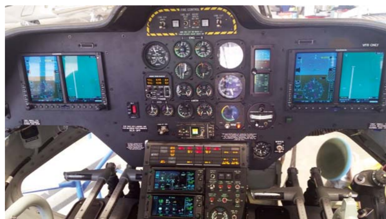
Garmin G600 and GTN650 installations by HAM Aero on a BK117 helicopter.
