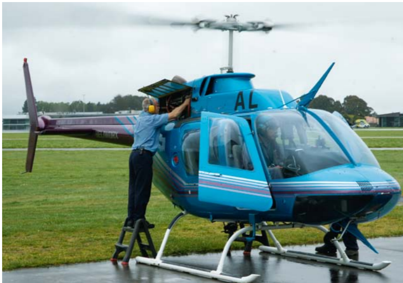
First run of Heliworx' JetRanger after a turbine refit following bearing replacement.
