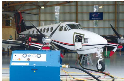
Tronair Cabin Pressurisation Unit being used to fault find pressurisation system in a King Air 300LW.
