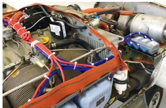
Electroair Electronic Ignition System fitted to turbocharged Continental. The first fitted to a Cessna 402B worldwide!
